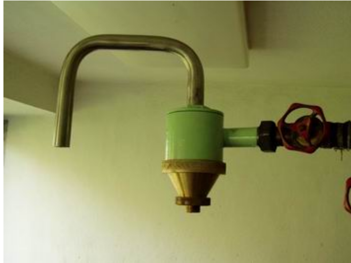
Fig. 5: Hydrocyclone with a 60° angle conical part
