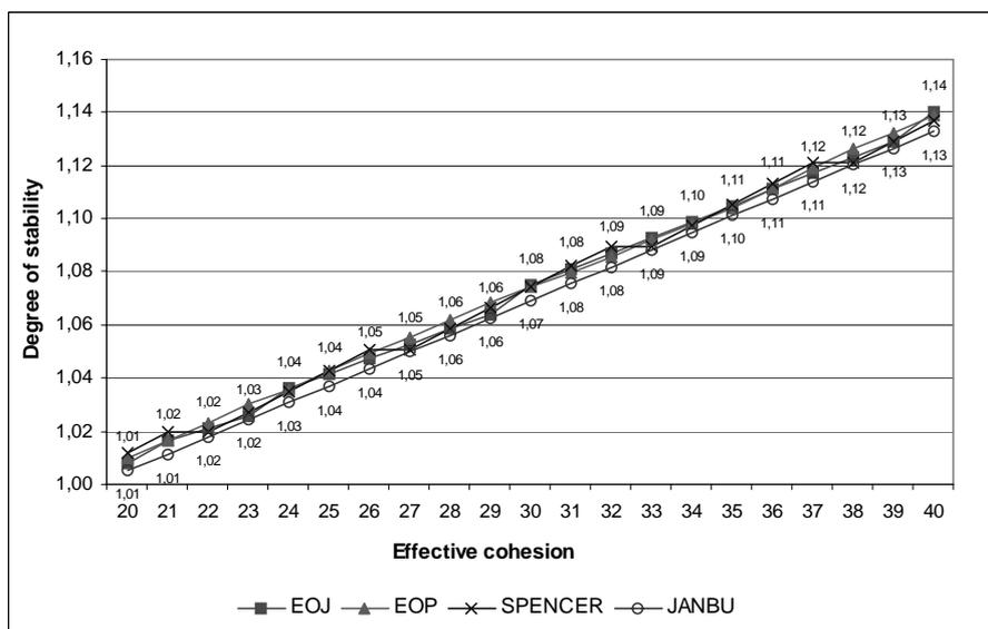
Graph 3: Dependence of stability degree on rising of effective cohesion of underlying bed with parameters: unit weight 21 [kN/m<sup>3</sup>]; effective angle of internal friction 25 [°]; saturation 1
