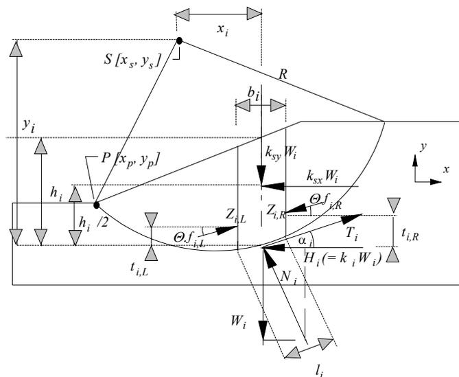
Fig. 1: Scheme of GeoStar methods
