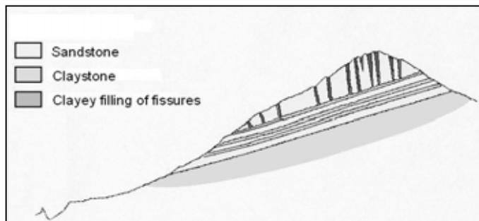
Fig. 2: Type model slope deformation
