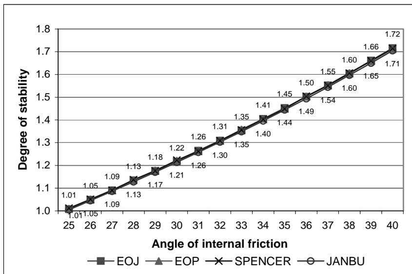
Graph 2: Dependence of stability degree on increase of effective angle of internal friction of underlying bed with parameters: unit weight 21 [kN/m<sup>3</sup>]; effective cohesion 20 [kPa]; saturation 1
