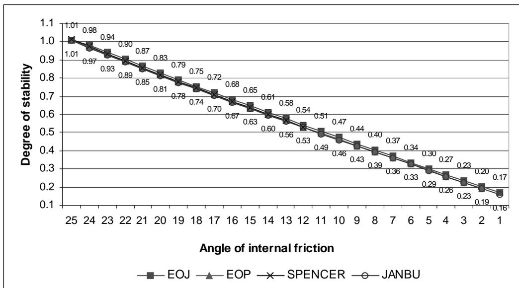
Graph 1: Dependence of stability degree on decrease of effective angle of internal friction of underlying bed with parameters: unit weight  $21 \text{ [kN/m}^3\text{]};$  effective cohesion  $20 \text{ [kPa]};$  saturation 1
