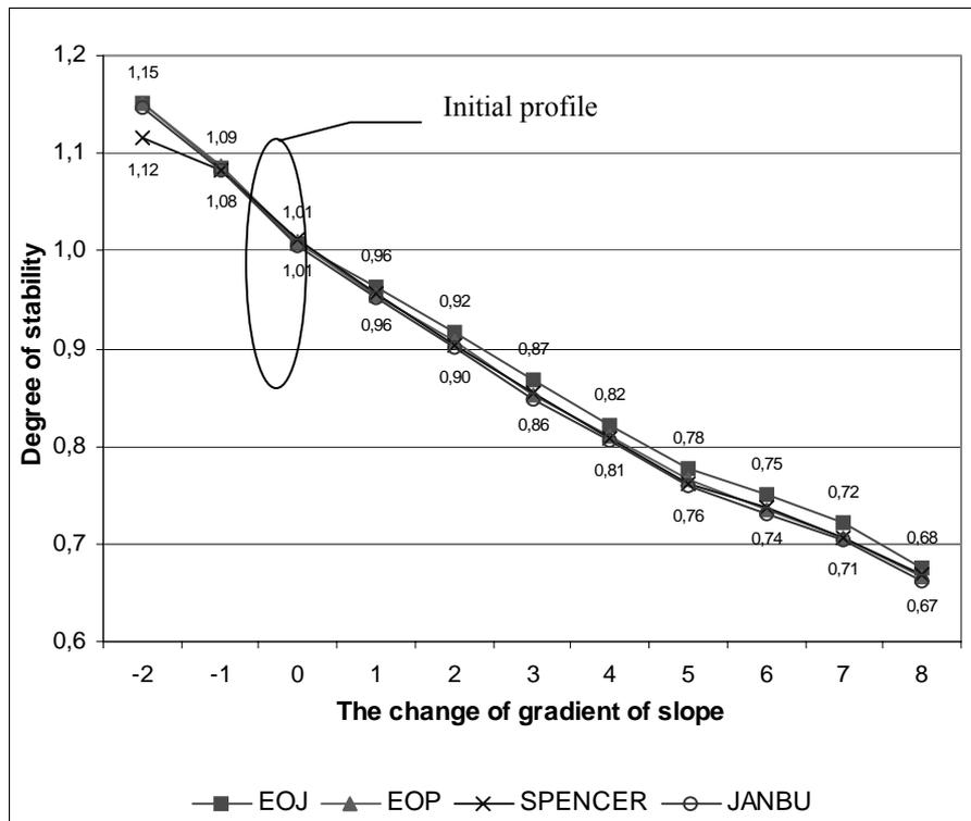
Graph 6: Dependence of degree of stability on the change of gradient of slope
