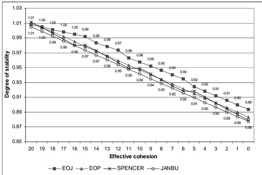
Graph 4: Dependence of stability degree on decrease of effective cohesion of underlying bed with parameters: unit weight 21 [kN/m<sup>3</sup>]; effective angle of internal friction 25 [°]; saturation 1
