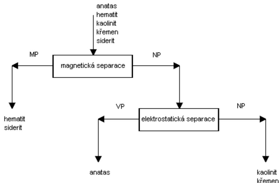
**Fig. 1** Flow diagram of the proposed separation process
