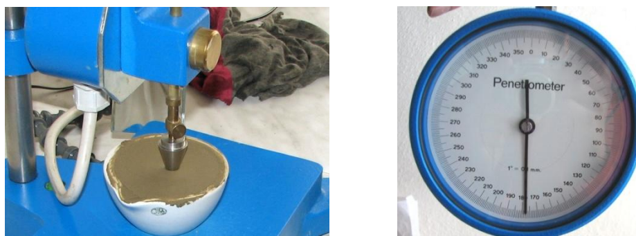
Fig. 2a (left) Cone test – cone sinking into paste Fig.. 2b (right) Penetrometer after sinking
