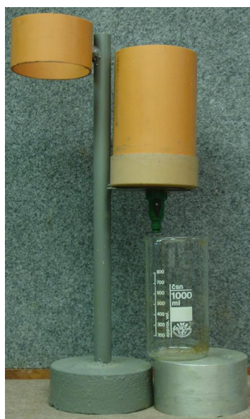
Fig. 2 Gravitational filtration testing apparatus (TARGF)
