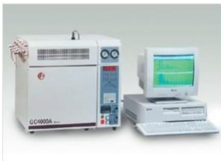
Fig. 7 Gas chromatograph GC-4008B designed for coal mines, [20].
