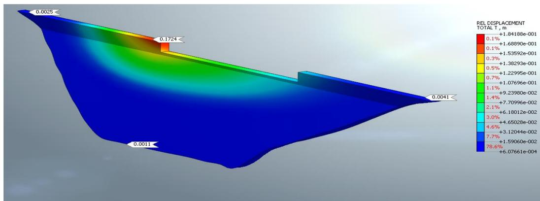
*Figure 13. Displacement at the end of the first earthquake*
