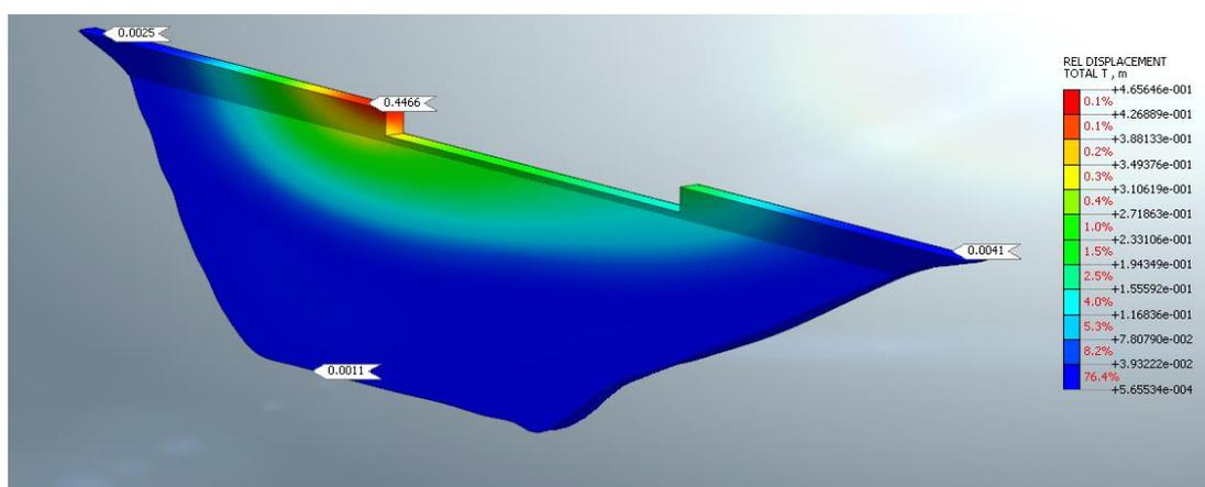
*Figure 14. Displacement at the end of the second earthquake*
