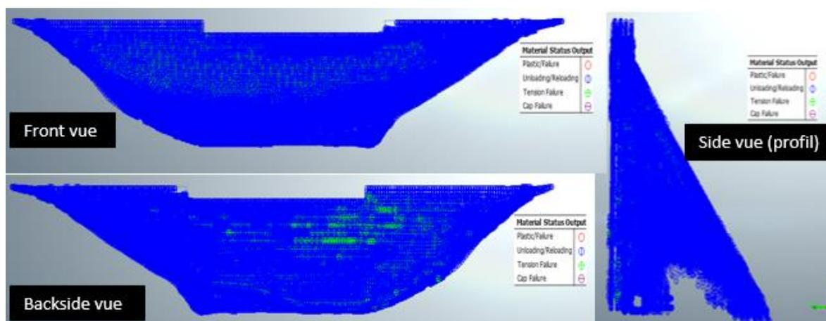
*Figure 15. Plasticity state of the first earthquake*
