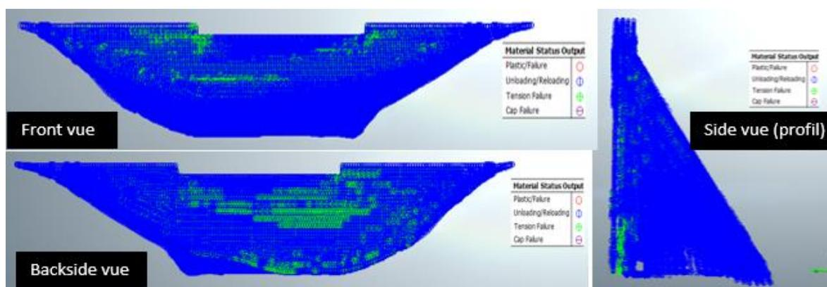
*Figure 16. Plasticity state of the second earthquake*
