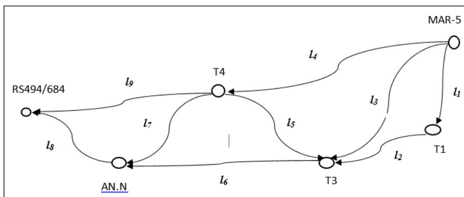
**Figure 4.** Levelling network
